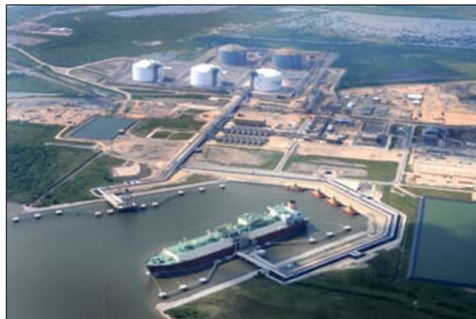
"Al Gharrafa" which sailed from Qatar to be the first Q-Flex to bring a cargo to the U.S. (Membrane containment - 216,000 cm capacity)
