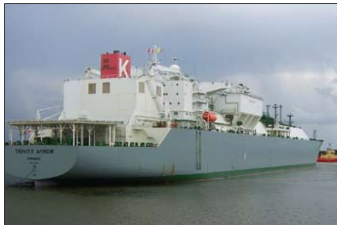
"Trinity Arrow" sailed from Nigeria to bring the third cargo to the Sabine Pass LNG Terminal. (Membrane containment - 154,000 cm capacity)
